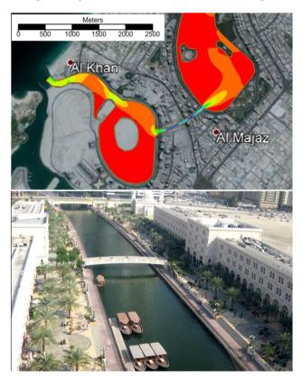
**Fig. 4** Simulation of the velocities and view of the Qasba canal, Sharjah, UAE (modeling and photo by the authors)
