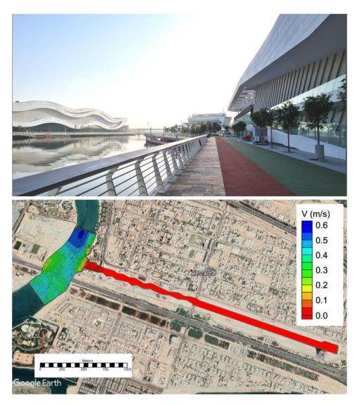
Fig. 5 Al-Qana (top). simulation of the velocities in the Qana canal (bottom)
